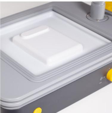
Both parts are formed from a PVC sheet and trimmed using a scalpel and a trim line
