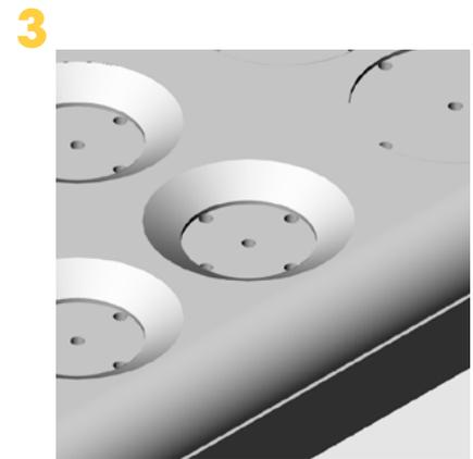
Holes are added to vent air out
