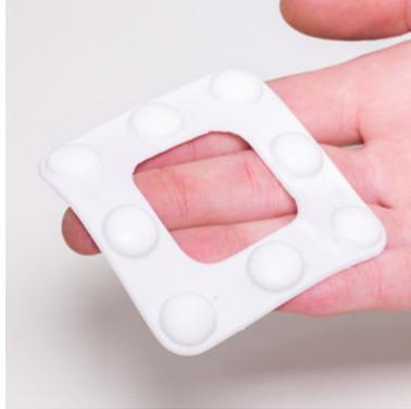
The silicone left to cure and removed from the mold
