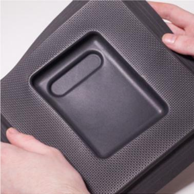
A sheet of EVA foam is formed around a slightly smaller template, this is done for both the front and back and trimmed at the seam line between the case shells
