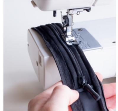
A zip is stitched into a loop with edges prepared so they join to case shells
