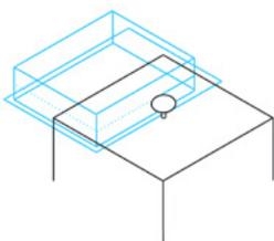
**Trimming edges with a form cutter**
