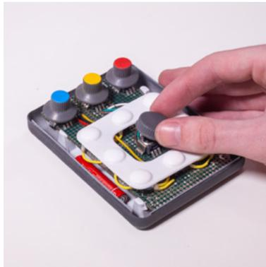
The dials are glued onto the potentiometers
