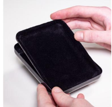
The tray is glued into the base and the cover is placed on top
