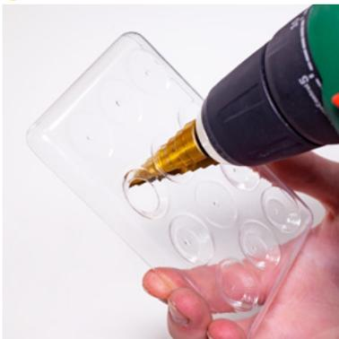
Holes for the various components are drilled out
