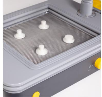
The inner and outer templates for the resin dials are formed with a polypropylene sheet
