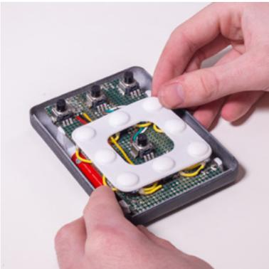
The silicone buttons are laid onto the switches
