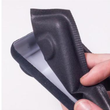
The EVA foam sheet is bonded to the inside of the PVC shells with contact adhesive
