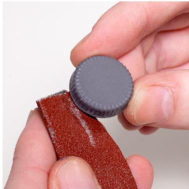
Any roughness or flash on the cast parts is sanded and polished
