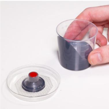
A durable plaster based resin is mixed with a pigment and cast in two stages to make dials with coloured caps
