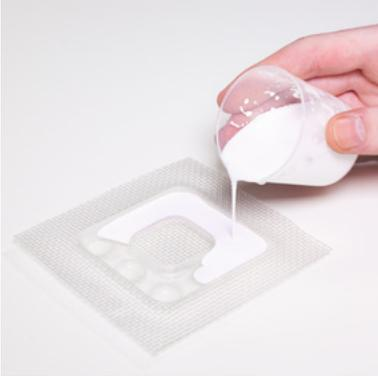
A medium shore-hardness RTV silicone is mixed with a pigment so it's translucent white and poured into the mold
