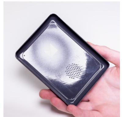
The shell's back is spray painted with frosting to diffuse the light from the LED behind
