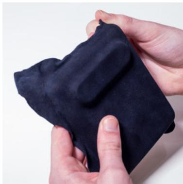
Napa leather is gently stretched around the PVC shells using a contact adhesive to bond the layers
