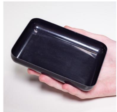
The base is formed using a black ABS sheet trimmed with a scalpel and a trim line
